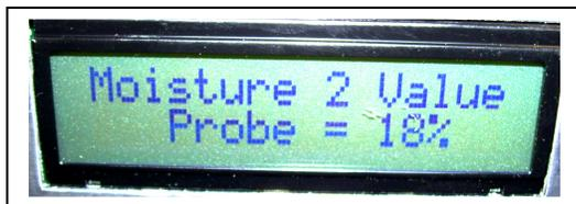
Press **SELECT** to set Moisture Probe shutdown percentage. Use **UP/DOWN** to change moisture percentage level set point.
