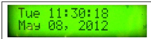
Press **SELECT** to set the E-TES SD Date & Time Clock. HOUR will flash first. Use the **UP/DOWN** buttons to change the HOUR setting. When correct, press **SELECT** to move to MINUTES, then SECONDS, MONTH, DAY NUMBER & finally YEAR. Use **UP/DOWN** to change each setting and **SELECT** to move to next option. When correct, press **SELECT** to save setting
