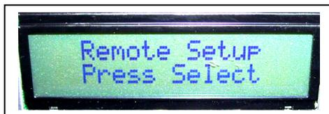
Press **SELECT** to set the E-TES Remote Exhaust Controller turn on temperature. Use **UP/DOWN** to change temperature.
