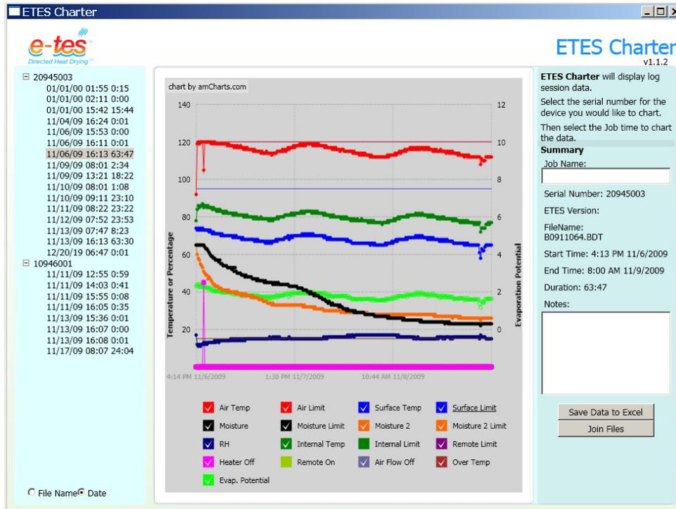
By moving your cursor over the graph it will display flags with the readings for individual points on the graph lines, as shown in the example below.
