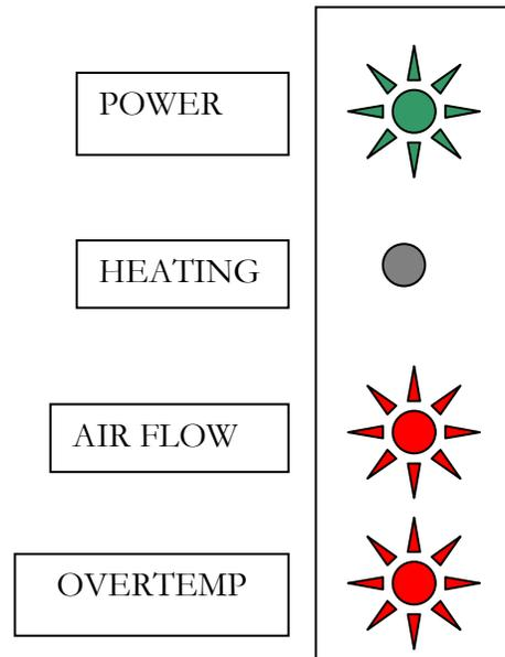
When the green **HEATING** light is OFF, but neither of the red lights is ON, it usually means that one on the remote sensors is getting a reading past its set point. When the AIR TEMPERATURE, SURFACE TEMPERATURE or MOISTURE VALUE measured by the corresponding probe exceeds the set point the green **HEATING** light will turn OFF indicating unit has shutoff the power to the heating elements.
