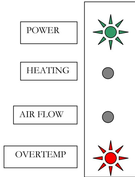
In some situations when the air flow is too low and the **AIRFLOW** light comes ON, the E-TES will also over heat and cause the **OVERTEMP** light to come ON too.
