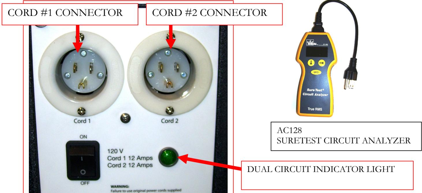
**With Cord #2 disconnected or connected to a dead outlet, as long as there is power to Cord #1 and Cord #1 is connected to the E-TES SD 120 Volt unit, the LED display and the POWER & HEATING indicator lights will still function, but the heater will only operate at one half of its rated heating capacity.**
