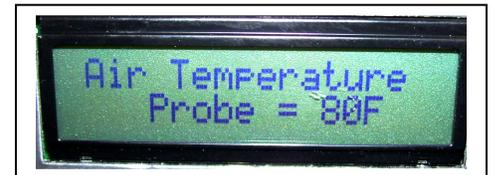
**Air Temperature Screen:** This tells you the current reading of the Air Temperature Sensor probe if it is connected to the E-TES SD or the default value of 00F if the probe is not connected.
