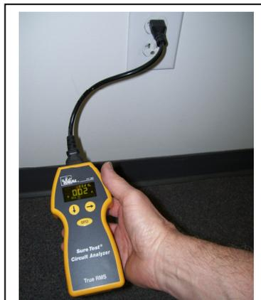
USE CIRCUIT ANALYZER TO CHECK CIRCUIT LOAD
