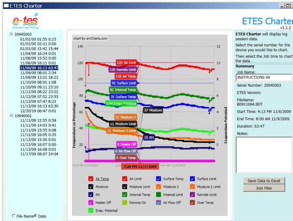
In this example of an Excel graph, you can see that the AIR TEMPERATURE LIMIT and REMOTE LIMIT were set at 120°F, the SURFACE TEMPERATURE LIMIT was set at 95°F, and the MOISTURE 1 LIMIT and MOISTURE 2 LIMIT were set at 15%. The RH or Relative humidity stayed around 15 to 20%. The INTERNAL TEMPERATURE stayed around 80-90°F. The E-TES unit never had the AIR FLOW turn off or an OVERTEMP condition.
