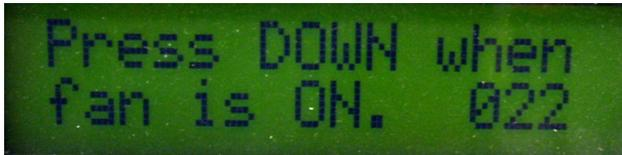
1. First turn the air mover OFF. When the fan is off and the number stops changing, press **DOWN**. This is the Off Set Point. (Shown as 000 in this example)
