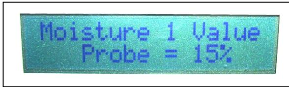
Press **SELECT** to set Moisture Probe shutdown percentage. Use **UP/DOWN** to change moisture percentage level set point.
