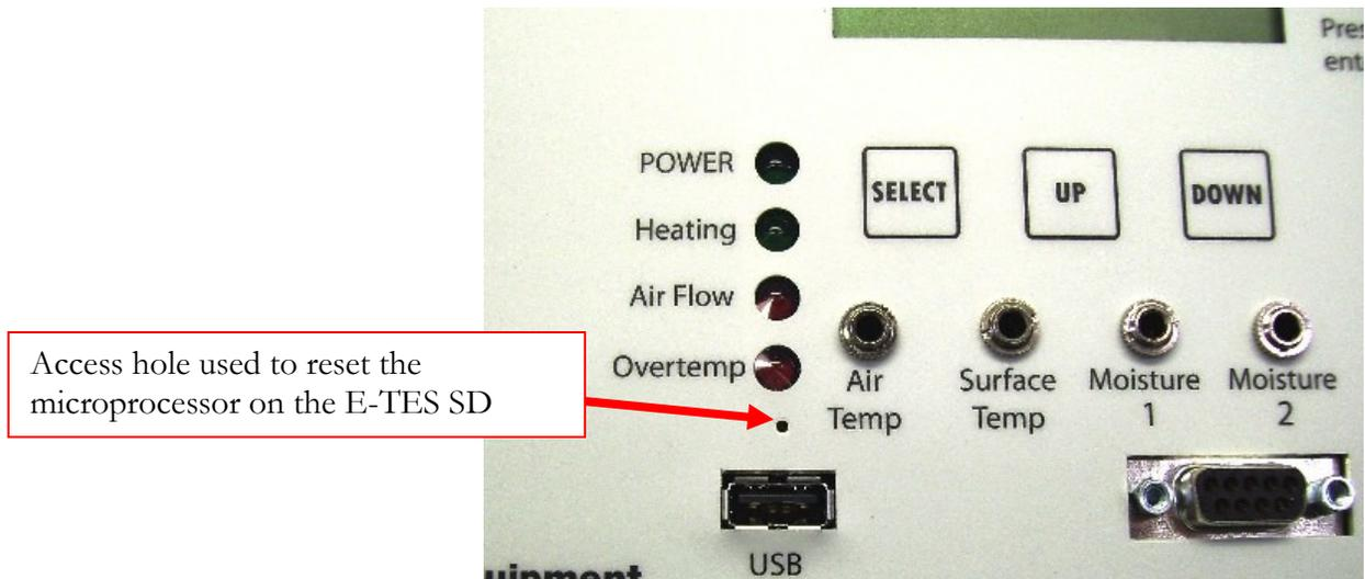
After resetting the processor, the E-TES SD Date & Time Clock must be reset.
