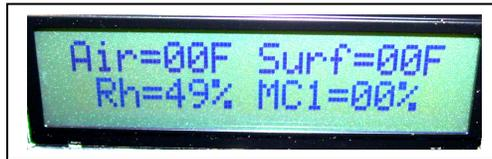
Main screen will display current probe temperatures or default settings if no probes are connected.
