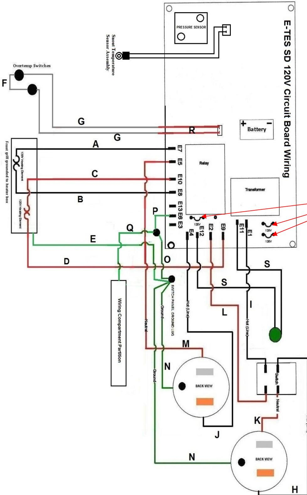
Three jumpers used to convert circuit board for use with 120vac must be in the positions shown for proper operation of E-TES SD unit.
