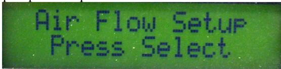
Press **SELECT** to set the Air Pressure Sensor trigger point. Follow the screen directions using the **DOWN** button to set the levels with the air mover OFF & ON.
