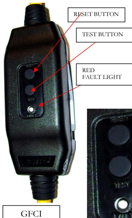
When the GFCI cord is connected to the 120vac outlet, push the RESET Button. Then, push the TEST button to test the GFCI.
